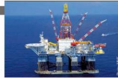
The Ocean Confidence semi-submersible rig is used to drill deep prospects in the deep-water Gulf of Mexico.
