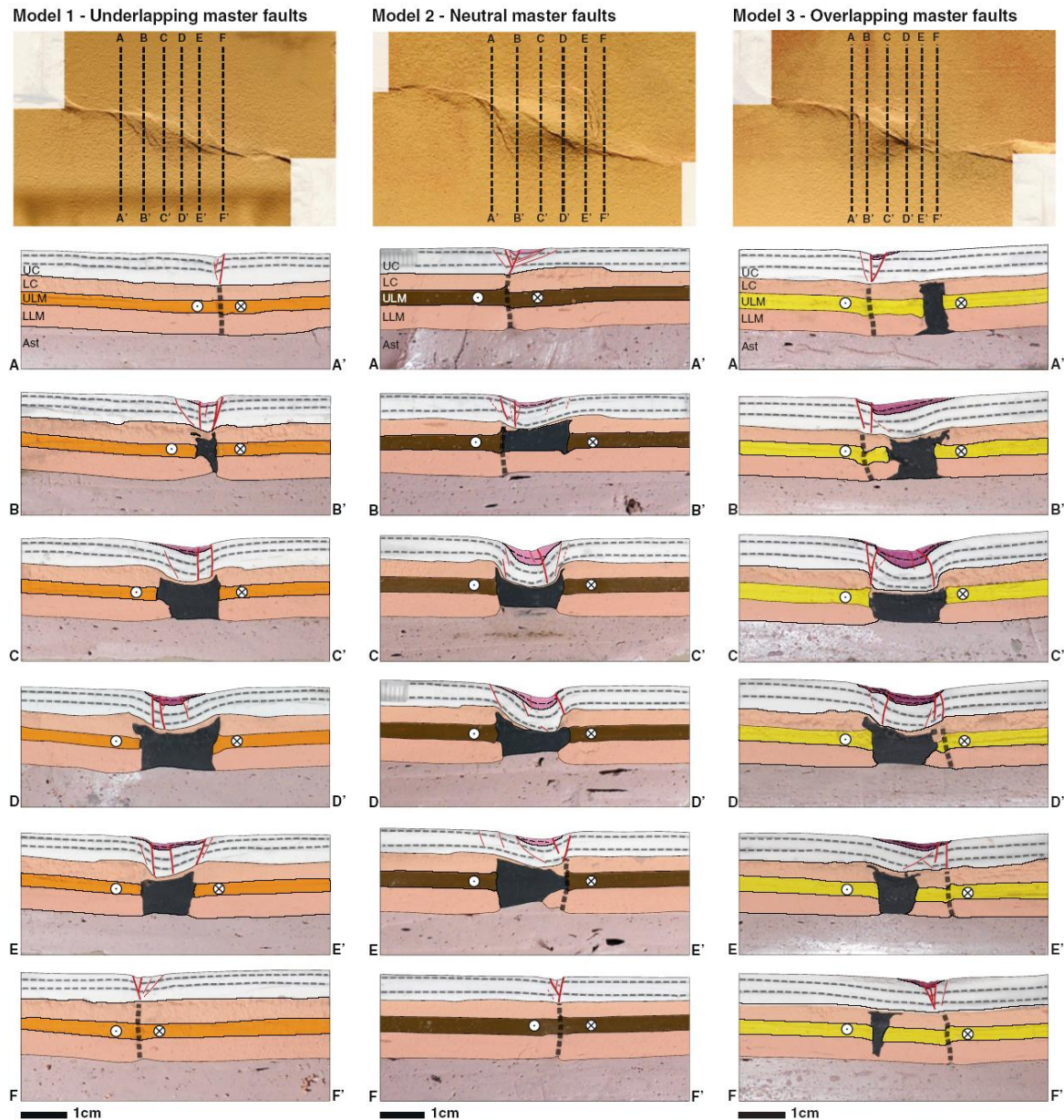
Fig. 6. Cross sections from the underlapping (left), neutral (centre) and overlapping (right) master-fault models. Of note is the along-strike variation in basin morphology and the dipolarity change from one end of the basin to the other. For example, in case of underlapping master faults, the upper crust dips mainly to the right in Section C-C' then flips to dominantly left dipping in Section E-E'. The same occurs in the other models. Note in sections B-B' and D-D' of Model 2 that the thin layer of lower crust above the black weak material composing the weakness zone has been in places completely removed by ductile thinning.
